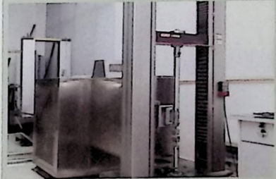
隔热型材抗剪切性能测试 thermal barrier strips anti-shearing property testing
